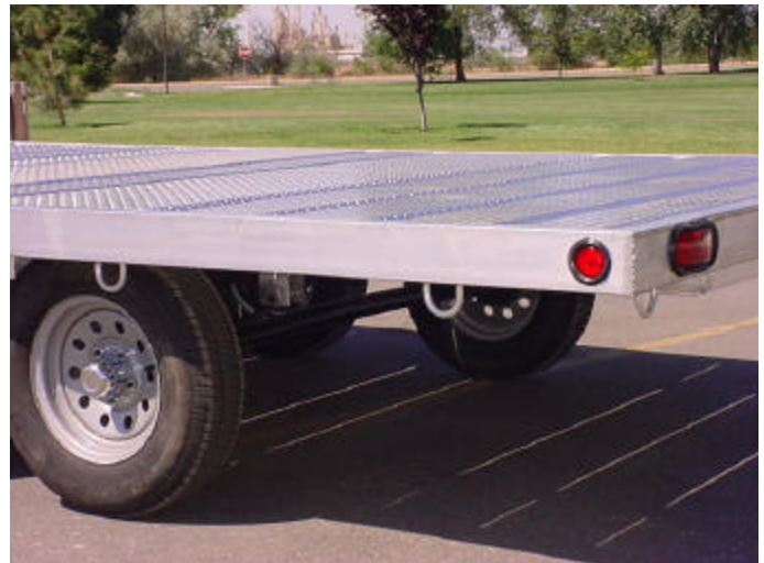
This trailer is complete with seal beam DOT lights, tie downs, and a slotted treadbrite deck to provide easy water run-off.
