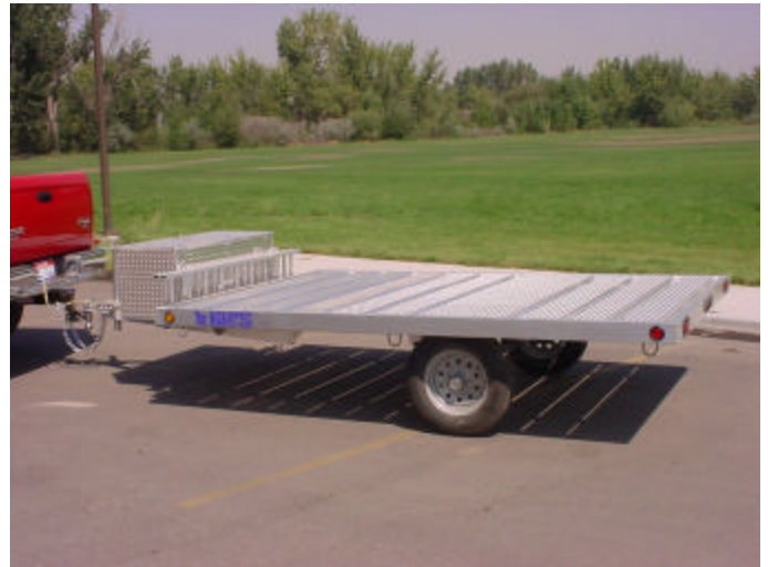
With 13" radial tires this trailer has a deck height of just under 27" off the ground for the easiest of loading.
